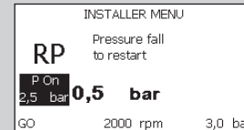
Figura 19: Setting the restart pressure
