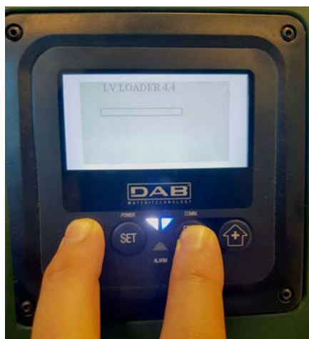
Figure 9C - Loader access for e.sybox
