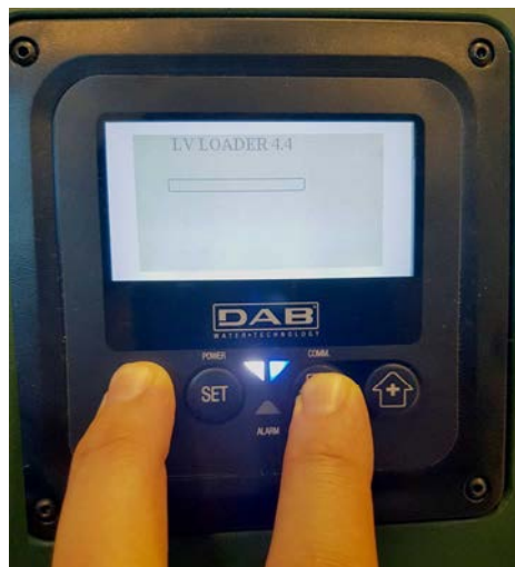
Figure 9D - Loader access for e.sybox mini3 Sw 1.X update
