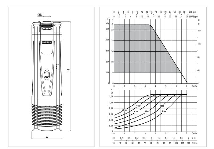
The performance curves are based on kinematic viscosity values =  $1 \text{ mm}^2/\text{s}$  and density equivalent to 1000 kg/m<sup>3</sup>. Curve tolerance according to ISO 9906.
