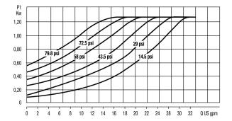
The performance curves are based on the kinematic viscosity values = 1 mm<sup>2</sup>/s and density equivalent to 1000 kg/m<sup>3</sup>. Curve tolerance according to ISO 9906.
