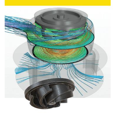
The new DAB patented Super Vortex impeller is redesigned to enhance performance of the FEKA FXV pumps under all conditions, reducing power consumption with free passage the same size as the pump's delivery port (2" and 2.5" / 50 and 64 mm).
