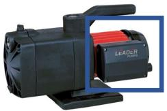
• The pumps must be filled with clean water (primed) before starting the pump. This can be done through the priming port. Do not run the pumps dry under any circumstance.
