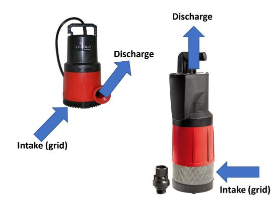
The Verty-Go's intake is on the bottom, and the discharge is on the top, but it has an integrated float switch. The float switch can be cleaned by pushing down on the float switch compartment handle, and pulling off the cover. It can be replaced by inserting the bottom of the float switch cover and snapping it closed by pushing it toward the pump.
