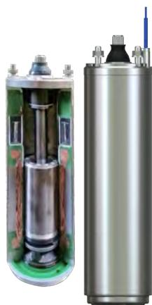
4" Asynchronous two-poles submersible motor, made in AISI 304 stainless steel for parts in contact with water. Cooling and lubrication of the thrust bearing assembly and carbon bushes is provided by a mixture of water and glycol. Squirrel-cage rotor mounted on Kingsbury self-centering thrust bearing. Stator housed in an airtight stainless steel casing (canned-type) with both flanges and shell in AISI 304L stainless steel.
