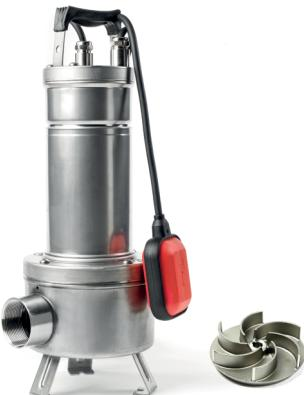
Submersible centrifugal pump with liquid vortex cast stainless steel impeller, suitable for pumping sewage water and waste water in general containing solids up to a maximum size of 2" (50 mm).
