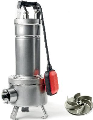
Submersible centrifugal pump with liquid vortex cast stainless steel impeller, suitable for pumping sewage water and waste water in general containing solids up to a maximum size of 2 in.
