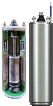
4" Asynchronous two-poles submersible motor, made in AISI 304 stainless steel for parts in contact with water. Cooling and lubrication of the thrust bearing assembly and carbon bushes is provided by a mixture of water and glycol. Squirrel-cage rotor mounted on Kingsbury self-centring thrust bearing. Stator housed in an airtight stainless steel casing (canned-type) with both flanges and shell in AISI 304L stainless steel.
