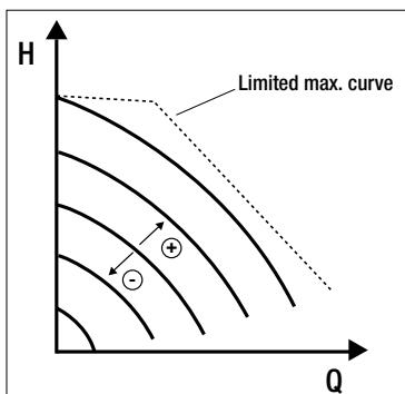
In this control mode, the circulator works based on constant speed characteristic curves. The operation curve is selected by setting the rotation speed using a percentage factor. The 100 % value indicates the maximum limit curve. The actual rotation speed may be affected by the power and differential pressure limitations of the actual circulator model. The rotation speed may be set using the display, or either a 0-10 V or PWM external signal.
