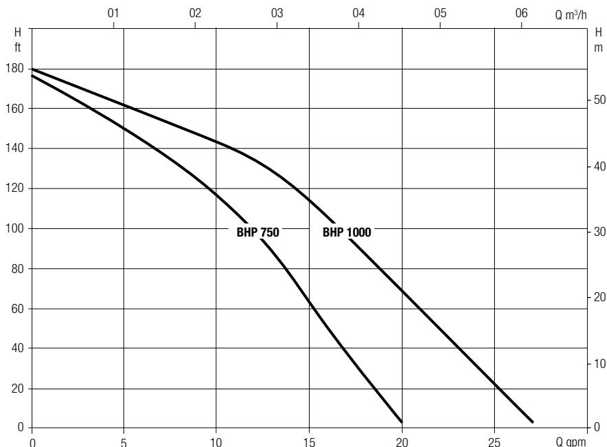
Curve tolerance according to ISO 9906.
