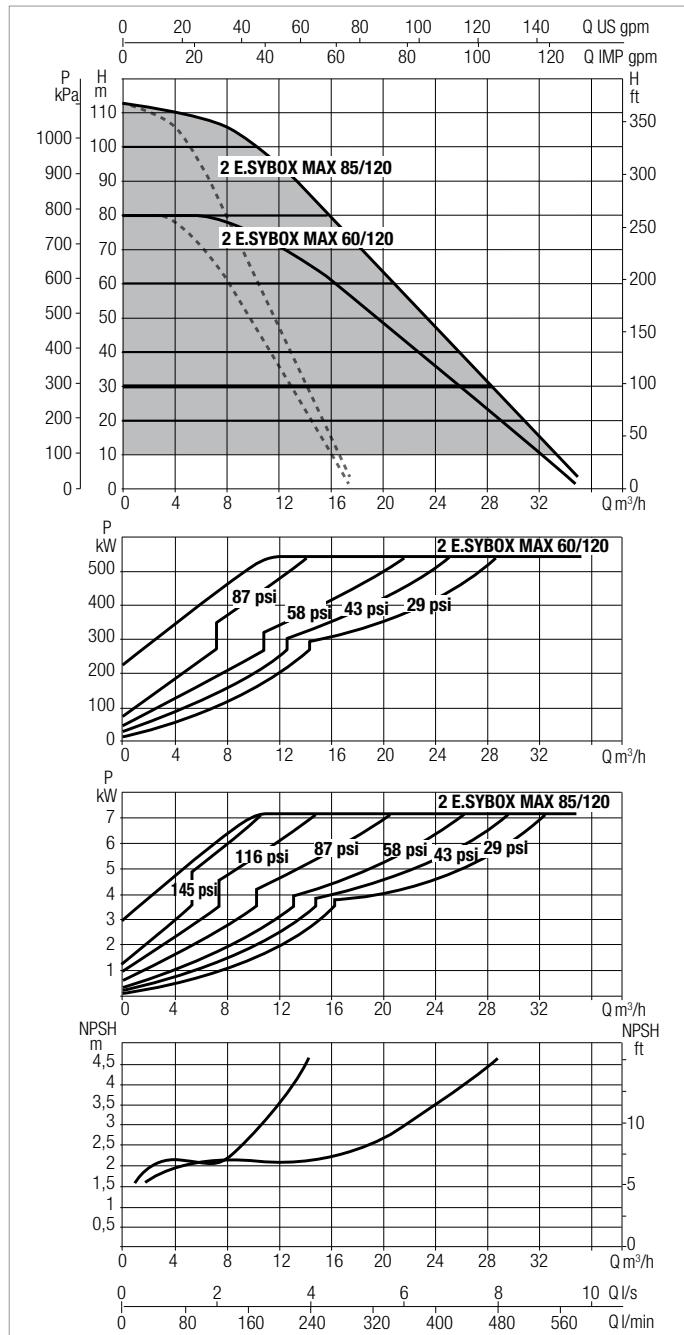
Curve tolerance according to ISO 9906.
