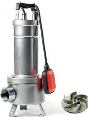
Submersible centrifugal pump with liquid vortex cast stainless steel impeller, suitable for pumping sewage water and waste water in general containing solids up to a maximum size of 2 in.
